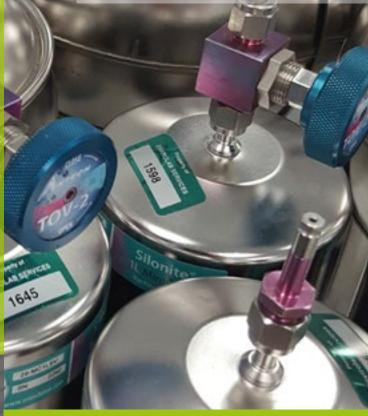
Canisters are used to test for volatile organic compounds (VOCs) in ambient air, indoor air, vapour intrusion, as well as soil and landfill gases.
